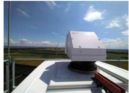
Gondola-mounted lidar on the wind turbine OPUS 1
