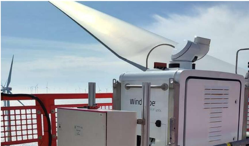
Scanning Lidar device on the nacelle of a wind turbine at RWE's offshore wind farm Amrumbank West. © Jörg Schneemann [2024]
