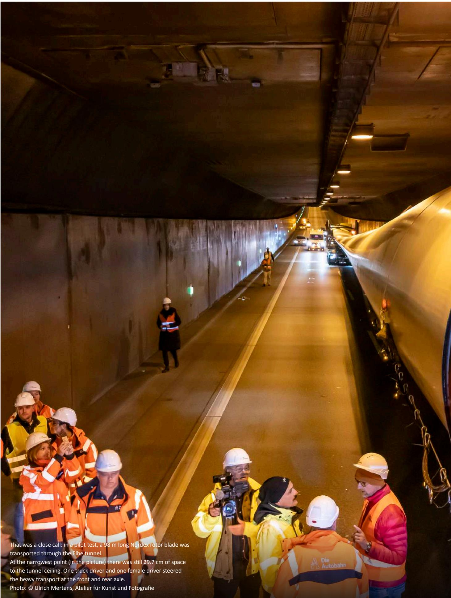
That was a close call: in a pilot test, a 98 m long Nordex rotor blade was transported through the Elbe tunnel. At the narrowest point (in the picture) there was still 29.7 cm of space to the tunnel ceiling. One truck driver and one female driver steered the heavy transport at the front and rear axle. Photo: © Ulrich Mertens, Atelier für Kunst und Fotografie
