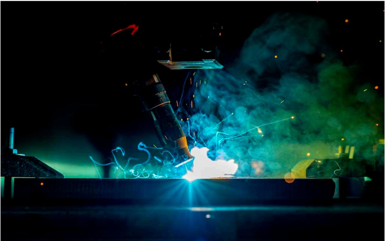
Laser hybrid welding using WeldMagnet from WeldNova GmbH during the process at 20kW laser power. © BAM
