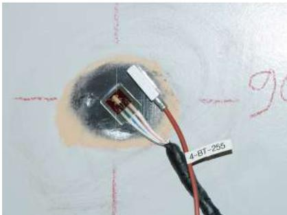
Recording the stresses of the steel tower by measuring the strains using strain gauges
