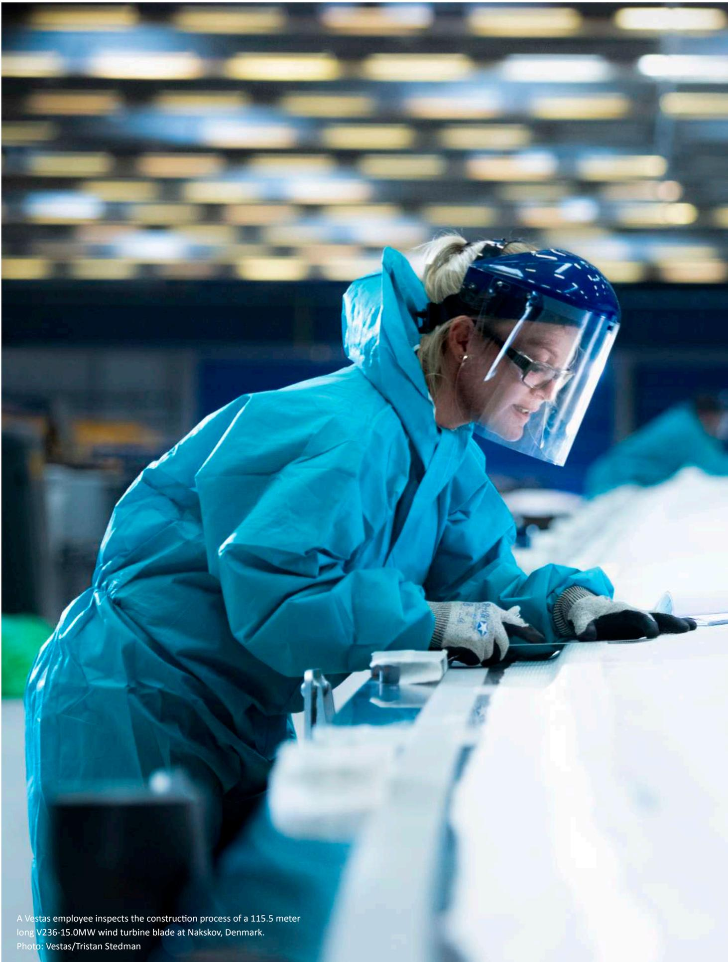
A Vestas employee inspects the construction process of a 115.5 meter long V236-15.0MW wind turbine blade at Nakskov, Denmark.
