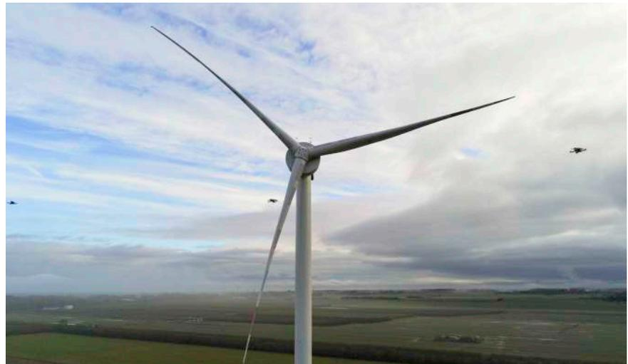
Drone fleet measuring the wake in front of the wind turbine OPUS 2
