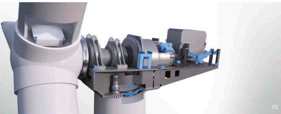
01 | Product portfolio in application from left: decoupling elements, cover mounts, yaw brakes, gearbox supports, TMDs, generator mounts, rolling mass absorbers
