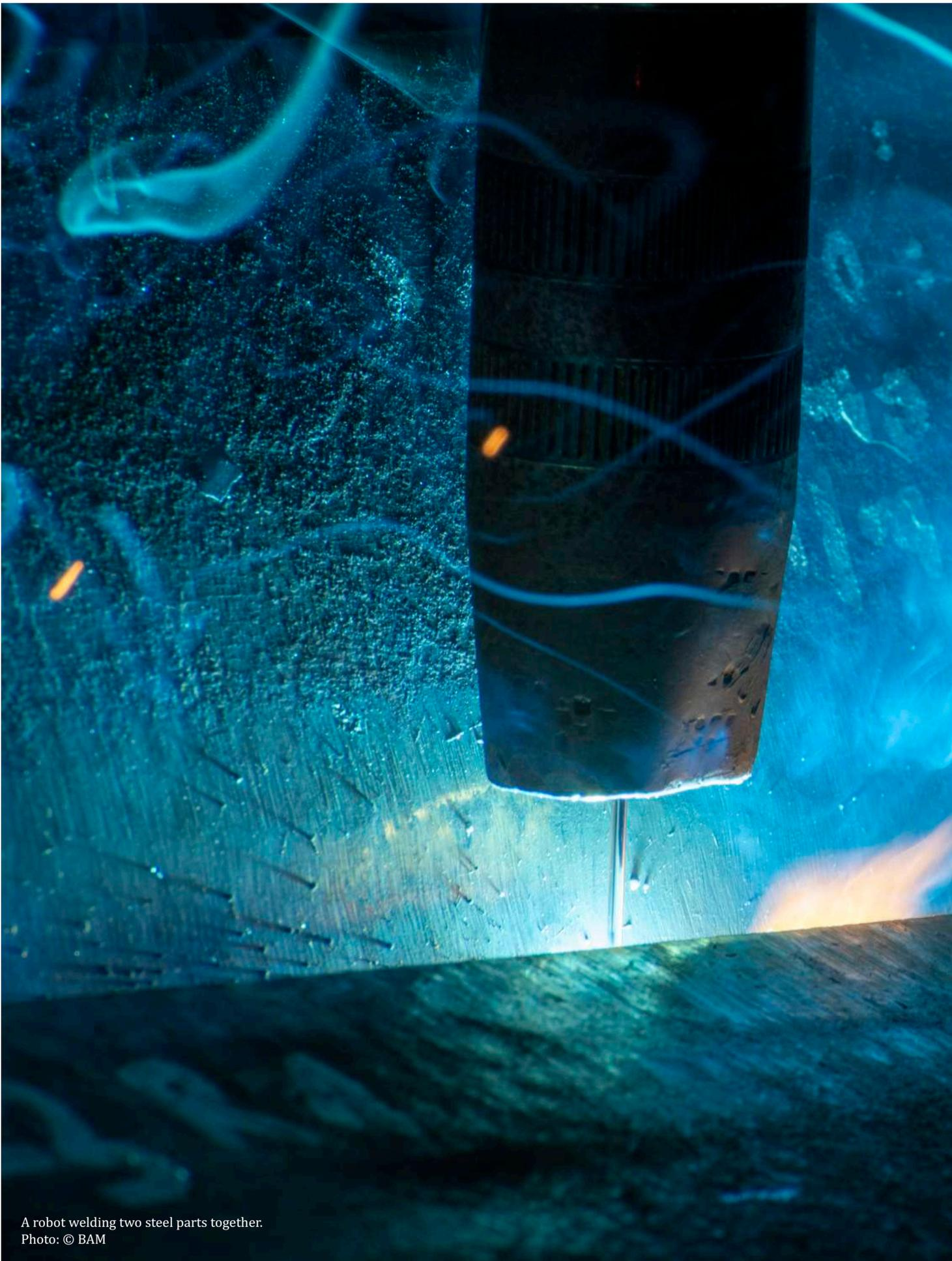
A robot welding two steel parts together.
