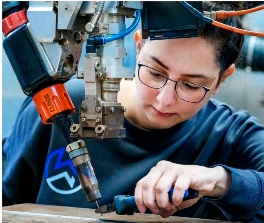
WeldNova technology makes laser hybrid welding a reliable and extremely efficient welding process for the wind industry. © BAM
