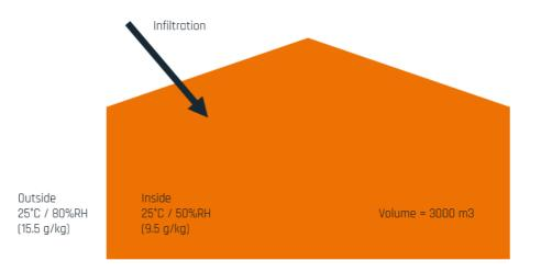
It is possible to determine the absolute water content in the air inside and outside from temperature and relative humidity by using the Mollier diagram. (see next page)
